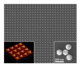
A plasmonic system modeling a trigonal planar molecule. The system consists of 142 nm-high gold nanodiscs with an 18 nm interparticle gap. Credit: A\*STAR
