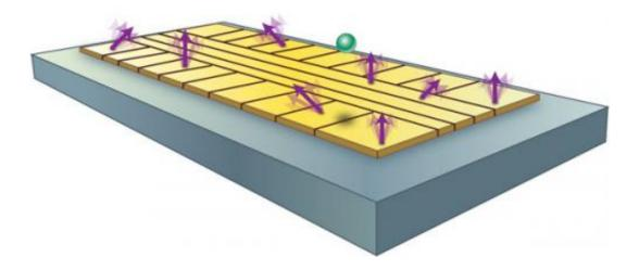
A schematic picture of a metal surface used in, for example, advanced detectors or quantum computers. New analysis has found that the excess noise levels seen in metal surfaces is caused by the thermal vibration of impurity atoms adsorbed onto the surface, shown here as purple arrows. (The green ball represents an ion part of the electrical device's operational mechanism - that has been intentionally placed on the surface. Credit: Physics Magazine
