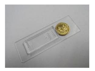
The Quake laboratory's MITOMI chip, designed for the rapid screening of molecular interactions, is providing a foundation for ongoing research at MSB. Credit: Bill Burkholder, MSB, IMRE, A\*STAR
