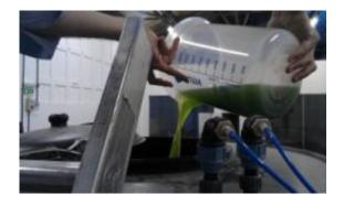
Algae is put into the photo bioreactor, which waste water will pass through. The algae will polish the waste water, and be harvested as a product.
