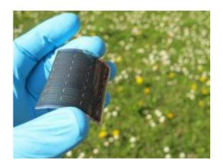
This is a flexible CIGS solar cell developed at Empa. Credit: Empa
