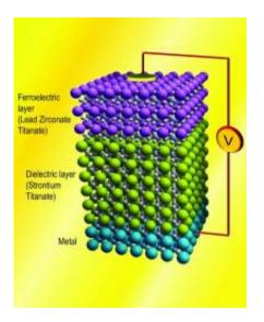
Shown is a rendition of an experimental stack made with a layer of lead zirconate titanate, a ferroelectric material. UC Berkeley researchers showed that this configuration could amplify the charge in the layer of strontium titanate for a given voltage, a phenomenon known as negative capacitance. Credit: Asif Khan, UC Berkeley
