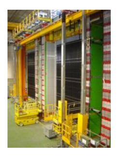
View of the OPERA detector (on the CNGS facility) with its two identical Super Modules, each one containing one target section and one spectrometer. Image: CERN
