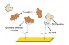
This is an expanded view of the aptamer-functionalized Surface Plasmon Resonance gold chip surface. Credit: University of Toledo
