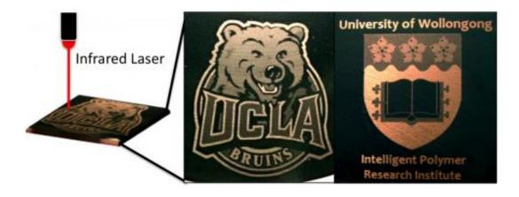
To demonstrate the high resolution of the patterning method, the researchers used the infrared laser to pattern the logos of UCLA and the University of Wollongong on disks. Image credit: Strong, et al. ©2011 American Chemical Society
