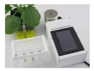
By detecting magnetic particles, the magnet reader can track down pathogens in plants. Filtration tubes are inserted into the reader for the purpose. ( $\bigcirc$  Fraunhofer IME)
