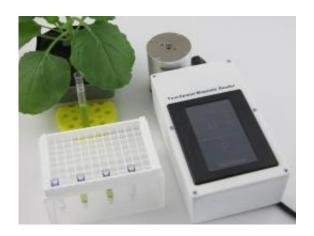
By detecting magnetic particles, the magnet reader can track down pathogens in plants. Filtration tubes are inserted into the reader for the purpose. (© Fraunhofer IME)
