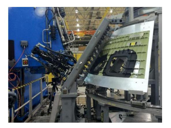
Construction on the first space-bound Orion Multi-Purpose Crew Module began with the first weld at the Michoud Assembly Facility on Sept. 9. 2011. This capsule will be used during Orion's first test flight in space. After welding is completed at Michoud, the Orion spacecraft orbital test article will be shipped to NASA's Kennedy Space Center, where the heat shield will be installed. At Kennedy, it will undergo final assembly and checkout operations for eventual flight. Credit: NASA
