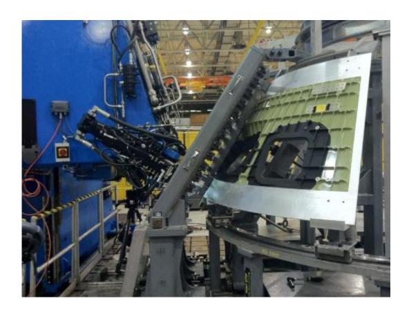
Construction on the first space-bound Orion Multi-Purpose Crew Module began with the first weld at the Michoud Assembly Facility on Sept. 9. 2011. This capsule will be used during Orion's first test flight in space. After welding is completed at Michoud, the Orion spacecraft orbital test article will be shipped to NASA's Kennedy Space Center, where the heat shield will be installed. At Kennedy, it will undergo final assembly and checkout operations for eventual flight. Credit: NASA
