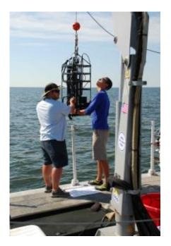
Scientists used multiple instruments to measure water quality. Here, members of the team deploy a package of instruments that take measurements of light interacting with particles in the water. Credit: Maria Tzortziou
