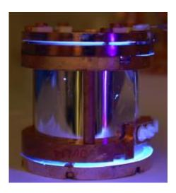
One of the CRESST detector modules. When illuminated with ultraviolet light, the scintillating inner shield glows brightly. Image: CRESST
