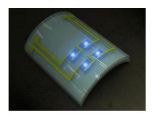
The team of professor Keon Jae Lee (Department of Materials Science and Engineering, KAIST) has developed a new concept: a biocompatible, flexible gallium nitride (GaN) LED that can detect prostate cancer. Credit: KAIST PR Office
