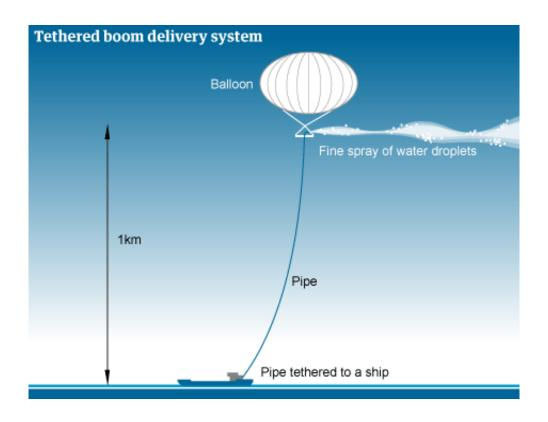
(PhysOrg.com) -- In what to some might seem almost ludicrous, (think Dr. Stranglove,) a British team of geo-engineers are set to launch a giant balloon a half mile into the sky pulling with it a water hose that will then spray water pumped from the ground, into the air. But this is only the beginning; the idea is to see if such a system is feasible. The real goal is to see if it might be possible to send such a giant balloon much higher,
