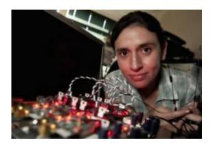
Rice University graduate student Melissa Duarte with a "full-duplex" test device. The technology, which allows wireless devices to "talk" and "listen" to networks on the same frequency, could double throughput on wireless phone networks. Credit: Jeff Fitlow/Rice University
