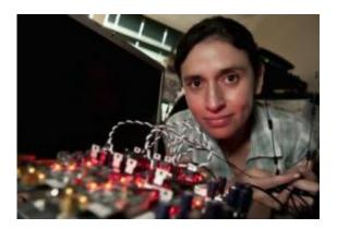
Rice University graduate student Melissa Duarte with a "full-duplex" test device. The technology, which allows wireless devices to "talk" and "listen" to networks on the same frequency, could double throughput on wireless phone networks. Credit: Jeff Fitlow/Rice University
