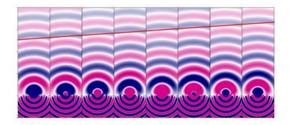
An array of nanoscale resonators, much thinner than a wavelength, creates a constant gradient across the surface of the silicon. In this visualization, the light ray hits the surface perpendicularly, from below. The resonators on the left hold the energy slightly longer than those on the right, so the wavefront (red line) propagates at an angle. Without the array, it would be parallel to the surface. Credit: Image courtesy of Nanfang Yu.
