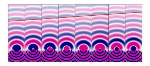
An array of nanoscale resonators, much thinner than a wavelength, creates a constant gradient across the surface of the silicon. In this visualization, the light ray hits the surface perpendicularly, from below. The resonators on the left hold the energy slightly longer than those on the right, so the wavefront (red line) propagates at an angle. Without the array, it would be parallel to the surface. Credit: Image courtesy of Nanfang Yu.
