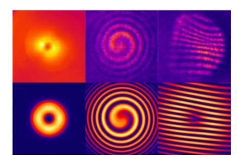
Nanfang Yu, Zeno Gaburro, Federico Capasso, and colleagues at SEAS have created strange optical effects, including corkscrew-like vortex beams, by reflecting light off a flat, nanostructured surface. The images at the top are experimental photos; the images at the bottom are simulations. Credit: Image courtesy of Nanfang Yu.
