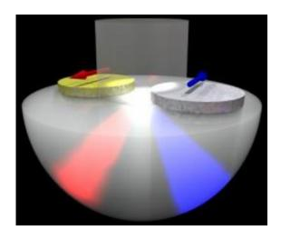
The nanoantenna acts as a router for red and blue light, due to the nanoparticles of gold and silver having different optical properties. Credit: Timur Shegai
