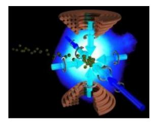
Illustration of the magneto-optical trap (MOT). The atoms (green spheres) are captured and cooled using three pairs of opposing laser beams (blue arrows) and a magnetic field generated by coils placed above and below the atoms. Credit: Niels Bohr Institute
