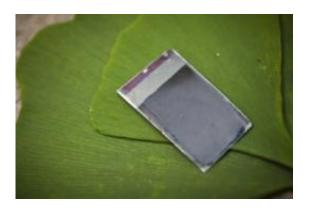
The 'artificial leaf,' a device that can harness sunlight to split water into hydrogen and oxygen without needing any external connections, is seen with some real leaves, which also convert the energy of sunlight directly into storable chemical form. Photo: Dominick Reuter
