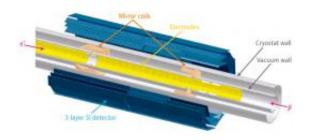
The ALPHA Collaboration's antihydrogen trap and detector. Antihydrogen is made when antiprotons (p) and anti-electrons (or positrons, e+) meet. The octupole (not shown) and mirror magnetic coils confine the antihydrogen, and a silicon (Si) detector records matter-antimatter annihilation events. Credit: Ref. 1 © 2011 ALPHA Collaboration
