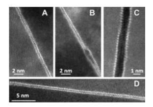
STEM HAADF micrographs show 2 layers of Bi absorbed along the general GBs of a Ni polycrystal quenched from 700°C. (C) Weakly bonded Bi atoms could cause the boundaries to easily fracture between layers and thus embrittle the material. Presumably, decohesion of this GB occurred during TEM specimen preparation. (D) A bilayer interfacial phase of similar character was observed in specimens quenched from 1100°C. Credit: Martin Harmer, Lehigh University
