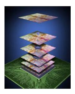
IBM and 3M Corp. are developing a new type of electronic "glue" that can be used to build stacks of semiconductors - 3D chips. The glue, shown in blue above, connects up to 100 separate chips as it conducts heat away from the silicon package. The innovation will create microprocessors 1,000 times more powerful than today's PC chips.
