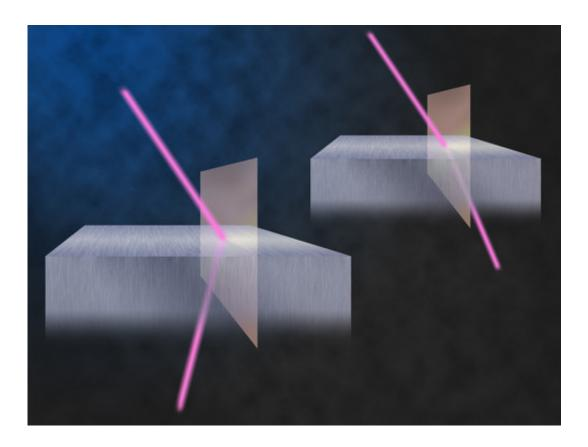
The beam of light enters the metal and is refracted into the opposite direction (left) compared to the usual behavior of light in materials (right).
