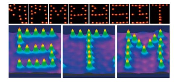
Letters drawn using an STM tip to move molecules. Electrostatic force between organic molecules (CH3S) and the STM tip was used to move the organic molecules to form the letters S, T and M (lower). The upper pictures show the drawing process for each letter. Copyright : RIKEN
