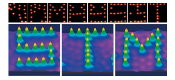
Letters drawn using an STM tip to move molecules. Electrostatic force between organic molecules (CH3S) and the STM tip was used to move the organic molecules to form the letters S, T and M (lower). The upper pictures show the drawing process for each letter. Copyright: RIKEN
