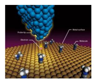
The principle of scanning tunneling microscopy. When a voltage is applied to an atomically sharp STM tip that is brought close to a molecule on a metal surface, a tunneling current flows between the tip and the molecule, injecting electrons into the molecule and inducing a molecular vibration. The intensity of the molecular vibration at a given voltage can be used to identify the molecule. This technique can also be used to induce a chemical reaction. Copyright: RIKEN
