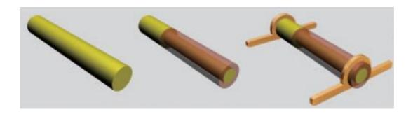
Schematic shows how to make core/shell nanowire solar cell starting from left with a CdS nanowire (green) that is dipped in CuCl where cation exchange reaction creates a Cu2S shell coating (brown). Metal contacts are then deposited on the CdS core and Cu2S shell. Credit: Image courtesy of Yang, et. al
