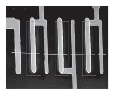
This scanning electron microscopy image shows three solar cells in series on a single nanowire with the core-shell regions marked by brown lines. Credit: Image courtesy of Yang, et. al
