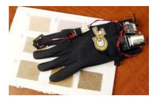
Georgia Tech researchers have developed a glove with a vibrating fingertip that improves tactile sensitivity and motor performance. The device uses an actuator made of a stack of lead zirconate titanate layers to generate high-frequency vibration to the side of the fingertip. Credit: Georgia Tech/Gary Meek
