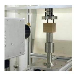
The ultrasound agitator causes the wood to vibrate, which generates frictional heat wherever there are cracks. A thermal imaging camera shows these defects up. (© Fraunhofer WKI)
