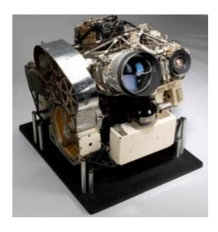
The Lunar Orbiter's onboard camera contained dual lenses that took photos
