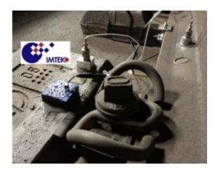
The power unit at the railway sleepers/ties in the Lotschbergbasis-tunnel in Switzerland can harvest enough energy to power wireless sensor nodes with a radio frequency interface. Image credit: M. Wischke, IMTEK
