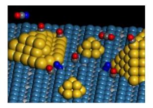
Image of a dual catalytic site causing the catalytic activation of an oxygen molecule (dark blue) at the perimeter of a gold nanoparticle held on a titanium dioxide support. A carbon dioxide molecule, produced by oxidation of adsorbed carbon monoxide, is liberated. Credit: Image by Matthew Neurock, University of Virginia
