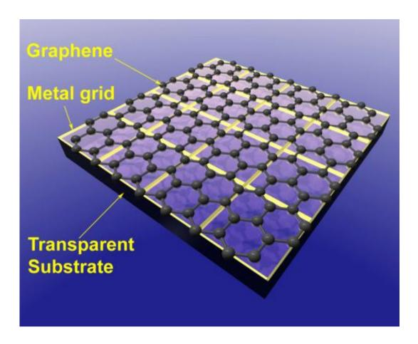
A hybrid material that combines a fine aluminum mesh with a single-atom-thick layer of graphene outperforms materials common to current touch screens and solar cells. The transparent, flexible electrodes were developed in the lab of Rice University chemist James Tour. (Credit: Yu Zhu/Rice University)
