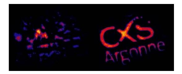
The impact of the new polyCDI technique is shown in these images of a twodimensional, 20-micron-wide gold test pattern reconstructed from coherent diffraction patterns taken with polychromatic X-rays. The left image was created using the conventional assumption that the X-ray beam consisted of a single wavelength; the right image used the new polyCDI algorithm takes into account a more-realistic spectrum of X-rays. Image courtesy Garth Williams.
