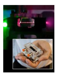
A laser pulse through a capillary filled with hydrogen plasma creates a wake that can accelerate an electron beam to a billion electron volts in just 3.3 centimeters. The same LOASIS accelerating structure has been modified to tune stable, high-quality beams from 100 to 400 million electron volts. Credit: Photos by Roy Kaltschmidt, Berkeley Lab Public Affairs
