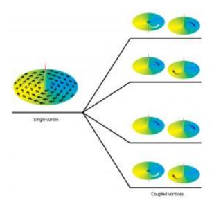
The magnetic domains in a single ferromagnetic disk arrange into a vortex (left). When two disks are brought close together (right), the magnetic vortices begin to move together. Their motion can be in-phase (bottom two levels), or out of phase (top two). The vortex cores can also point in the same direction, or in opposite directions, leading to four possible types of coupled motion. Credit: 2011 American Physical Society
