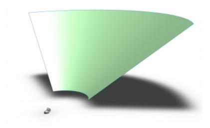
Diagram shows the idealized arrangement of a vat of molten salt used to store solar heat, located at the base of a gently-sloping hillside that could be covered with an array of steerable mirrors all guided to focus sunlight down onto the vat. Image: Courtesy of Alexander Slocum et al.
