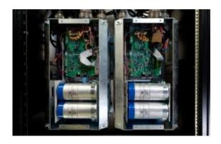
Two 50 kW Power Block prototypes with covers removed. Each power block consists of IGBT switches, a gate driver circuit, DC bus film capacitors, current sensors, DC bus voltage sensor, a heat sink temperature sensor, a digital controller board, bussing and connectors - all mounted on an air-cooled heat sink. Credit: Dennis Schroeder
