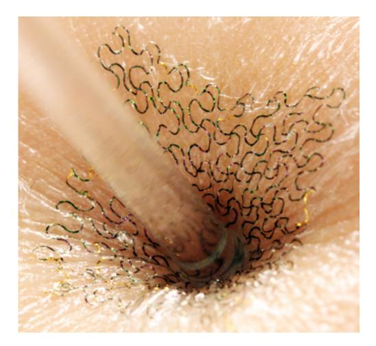
The circuits' filamentary serpentine shape allows them to bend, twist, scrunch and stretch while maintaining functionality. Photo courtesy John Rogers
