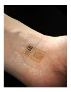
An ultrathin, electronic patch with the mechanics of skin, applied to the wrist for EMG and other measurements. Photo courtesy John Rogers
