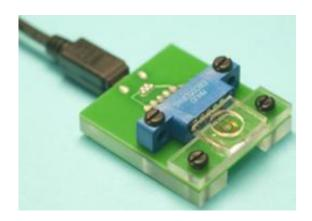
UC researchers have developed the first lab-on-a-chip sensor to provide fast feedback regarding levels of the heavy metal manganese in humans. The first field test of the sensor will be in 2012. Credit: Dottie Stover, University of Cincinnati
