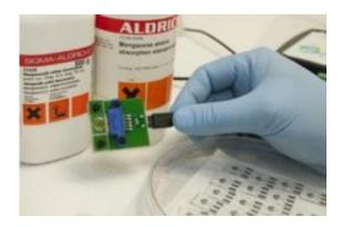
UC researchers have developed the first lab-on-a-chip sensor to provide fast feedback regarding levels of the heavy metal manganese in humans. The sensor is both environmentally and child friendly, and will first be field tested in Marietta, Ohio, where a UC researcher is leading a long-term health study on the potential health effects of heavy metals. Credit: Dottie Stover, University of Cincinnati
