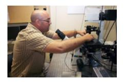
UW researcher Jay Gatlin prepares the machine that inserts microscopic probes into a cell spindle to measure the forces of the inward and outward pulls on microtubules, which act as structural elements like trusses and beams in a building. The probes are manipulated by joysticks. Credit: UW Photo
