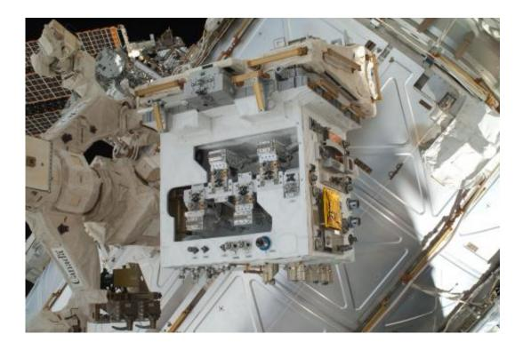
The Robotic Refueling Mission module, installed on its temporary platform on the International Space Station's Dextre robot. RRM will demonstrate robotic servicing technology and lay the foundation for future missions. Credit: NASA
