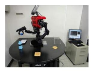
Researchers with the Hasegawa Group at the Tokyo Institute of Technology have created a robot that is capable of applying learned concepts to perform new tasks. Using a type of self-replicating neural technology they call the Self-Organizing Incremental Neural Network (SOINN), the team has released a video demonstrating the robot's ability to understand it's environment and to carry out instructions that it previously didn't know how to do.
