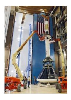
Engineers attach a collar to the escape vehicle on the Orion spacecraft at the Lockheed Martin facility in Denver on Friday, Aug. 12, 2011. They will use it to move the assembled craft to the testing chamber at left where it will be submitted to vibration testing. (AP Photo/Ed Andrieski)
