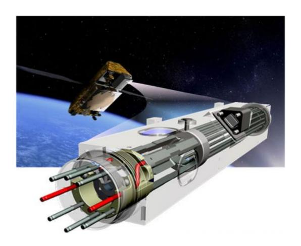
The device 'swooshing' into a satellite is the vacuum tube, one of the main components of an atomic clock that will undergo a technology flight demonstration.
