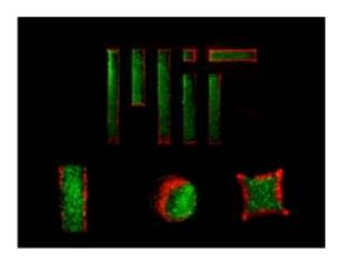
Using a temperature-responsive micromold, MIT engineers created two-layer gel microparticles (the red and green areas represent separate layers). Photo: Halil Tekin
