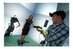
UCSD's Daniel Tenedorio in the middle of making a freehand 3D scan of Tiffany Fox in Calit2's StarCAVE using a modified Kinect. Though Fox's avatar appears to be projected onto the wall behind her, the scan is actually projected in the middle of the StarCAVE.
