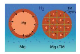
Particles of pure magnesium (left) can only collect a limited amount of hydrogen on their outer surfaces, and the process is slow. But when the magnesium is doped with iron (right), far more hydrogen is delivered through the iron layers, which also results in much faster charging. Credit: NIST
