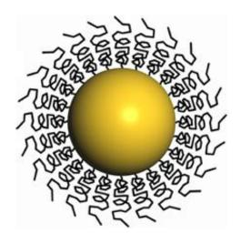
A schematic diagram shows a gold nanoparticle stabilized with polyvinyl alcohol (PVA) ligands.
