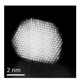
A micrograph taken by Lehigh's high-angle annular dark field (HAADF) scanning transmission electron microscope (STEM) shows a gold nanoparticle on a TiO2 support after a hot water wash.
