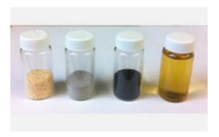
Vials containing sawdust, catalyst, charred catalyst and gasoline made from sawdust. Credit: Robert Coolman, UMass Amherst
