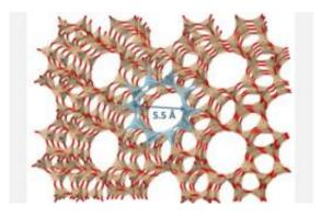
Structure of zeolite in a catalyst. Each tetrahedron represents either SiO2 (silicon dioxide) or HAIO2 (hydrogen aluminum dioxide). The spaces in the structure (highlighted) are called "micropores" and are roughly the same size as gasoline molecules. Credit: Image courtesy of the University of Wisconsin-Madison Materials Research Science and Engineering Center
