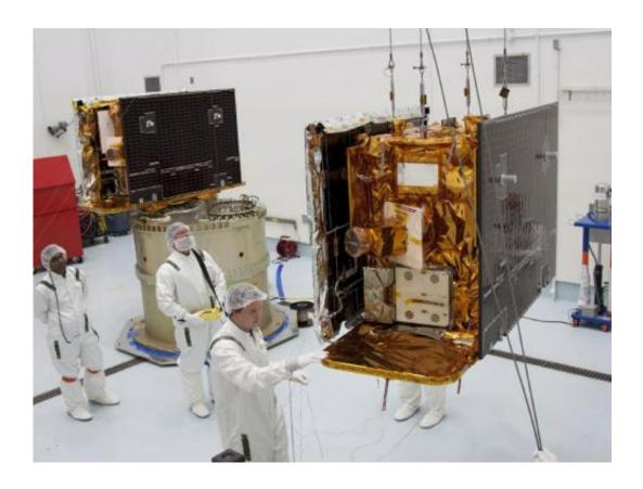
At Astrotech Space Operation's payload processing facility in Titusville, Fla., NASA's Gravity Recovery and Interior Laboratory-A (GRAIL-A) lunar probe is lifted from its workstand and across the clean room toward the spacecraft adapter ring, at left, where GRAIL-B is already secured. (8/10/2011)Credit: NASA/KSC
